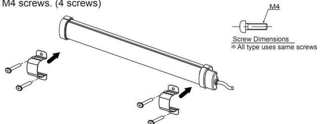
\*Holding bracket: 2incl for all types(CWA3S,CWA6S,CWA9S).
